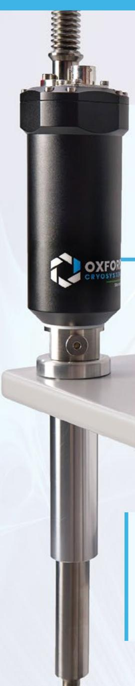
Eliminate the need for liquid nitrogen with this mechanically cooled open-flow system. The Cobra delivers the same cooling performance, temperature stability, and OEM integration as the Cryostream, but uses a closed helium circuit. This cryogen-free system features a smaller, lighter gas head and can operate continuously, providing reliable sample cooling day and night for automated, batch, and screening work-flows.
