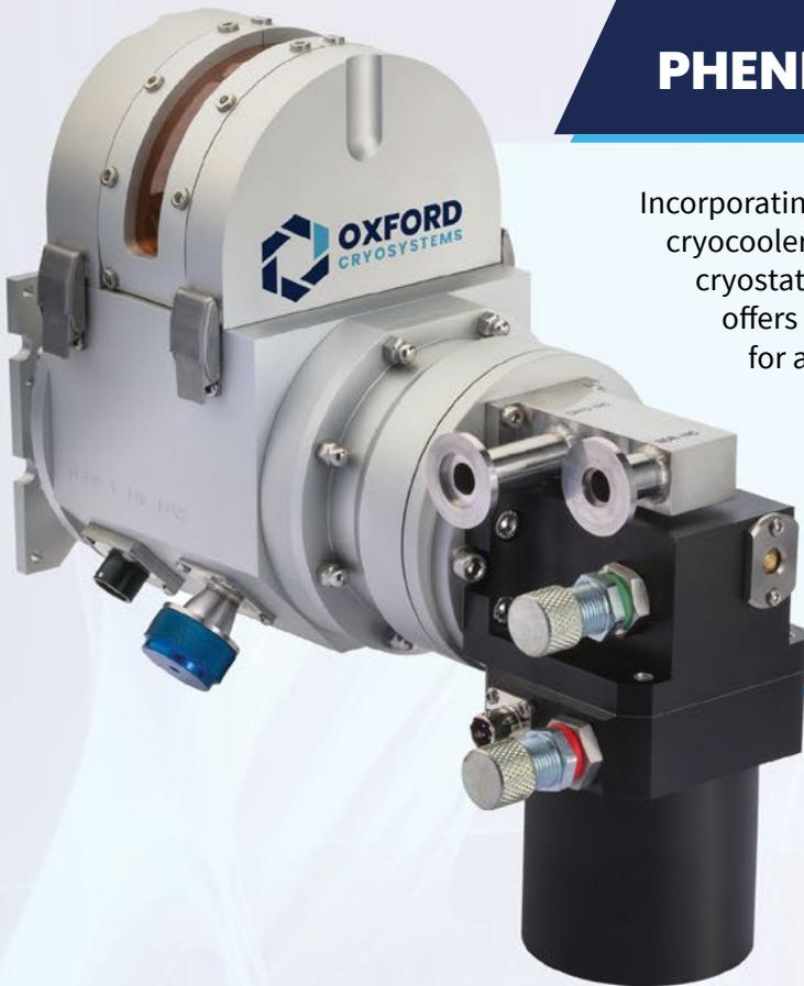
Incorporating our proprietary two-stage Gifford McMahon (GM) cryocooler, the Phenix is a closed-circuit sample-in-vacuum cryostat. Originally designed for powder diffraction, it offers excellent temperature stability from 12 K to 320 K for a broad range of applications.
