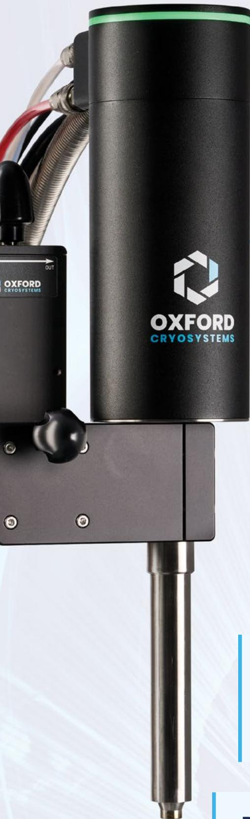
The universal standard for most diffractometers, this open-flow cooler enables diffraction studies for a range of applications, such as macromolecular structures and drug-protein interactions.
