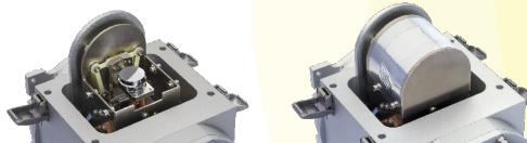
Heat leaks are reduced by a mylar radiation shield, while the PheniX lid includes X-ray transparent windows made of Kapton.
