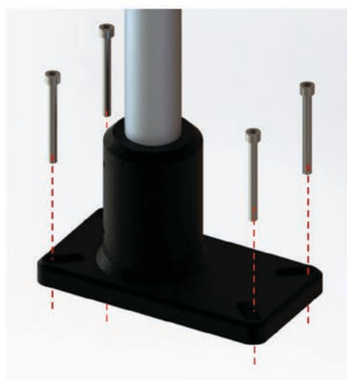
Figure 6.4 Schematic of varibeam base plate
