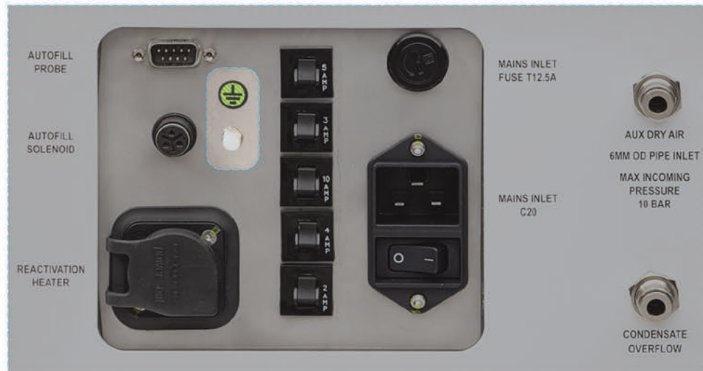
Figure 6.8 Earthing Stud Location
