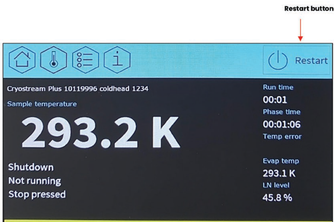
Figure 7.10 Home screen when Cryostream is stopped
