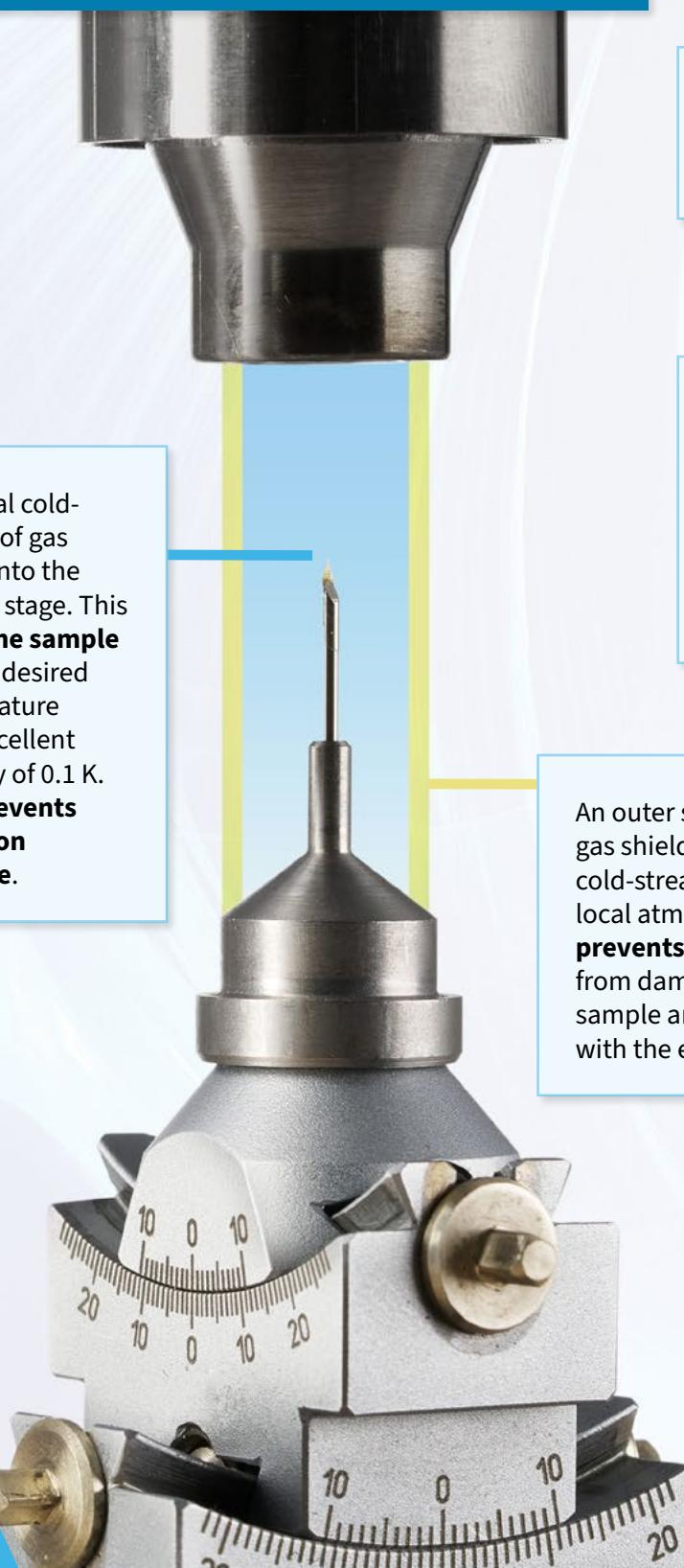
A central cold-stream of gas flows onto the sample stage. This **cools the sample** to your desired temperature with excellent stability of 0.1 K. This **prevents radiation damage**.
