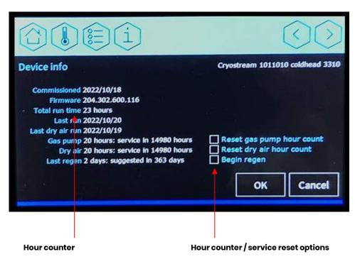
Figure 8.1 Device info screen showing the hour counter
