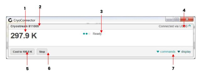
Figure A2: CryoConnector showing Overview Section only
