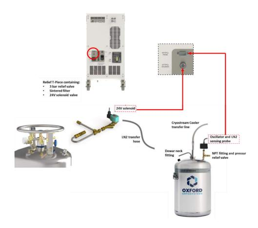
Figure A10 Schematic of autofill assembly
