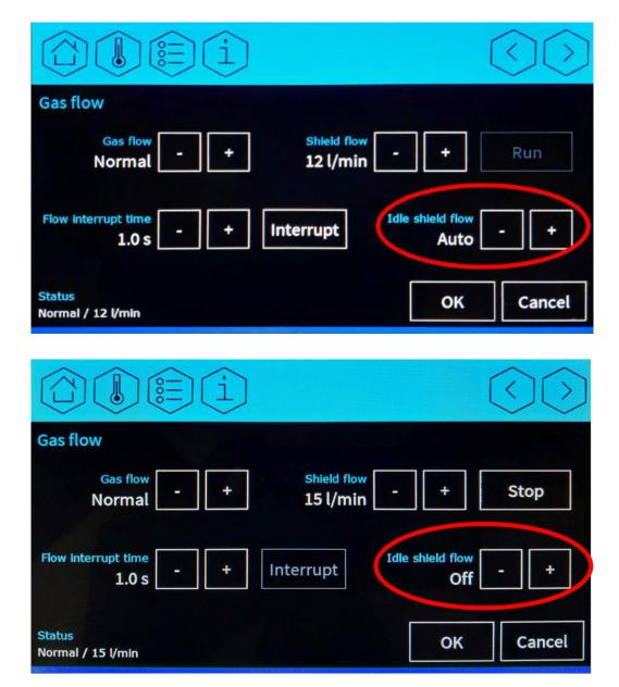
Figure 7.8 Idle Shield flow settings on the controller
