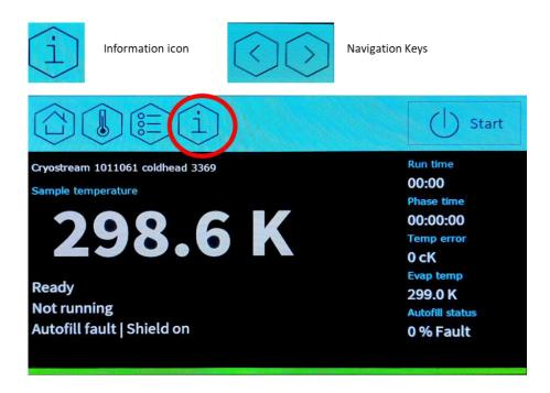
From the home page, navigate to the relevant screens using the information icon (displayed above) and then navigate to the relay board diagnostic screen, the live diagnostic screen and the flow diagnostic screen. Take photos of these and attatch them to an email to <a href="mailto:support@oxycryo.com">support@oxycryo.com</a> along with the serial number of the GSM and Coldhead. See below the relevant images to send:
