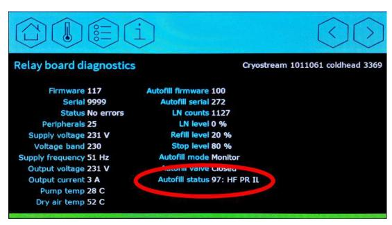
Figure A14 Accessing the autofill status from the live diagnostic screen or the Relay board diagnostic screen
