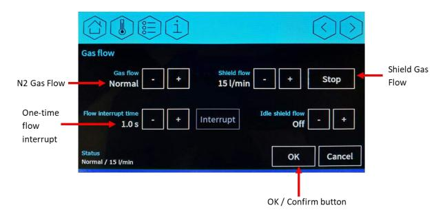
Figure 7.12 Command screen 2 showing gas flow settings
