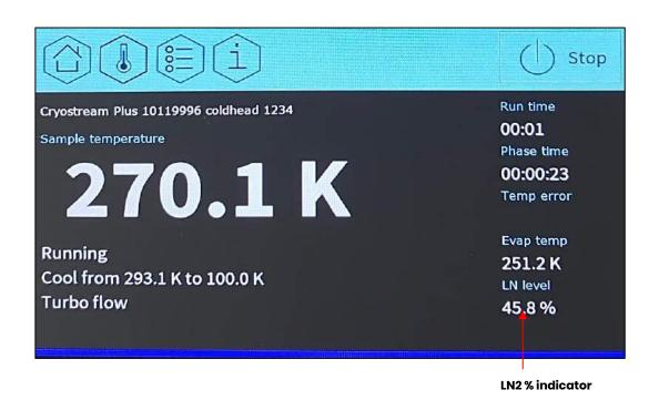
Figure A11 Location on screen of liquid nitrogen level
