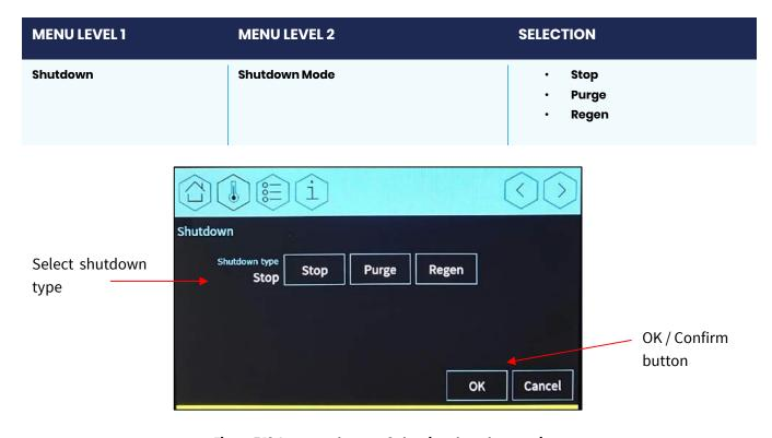
Figure 7.13 Command screen 3 showing shut-down options
