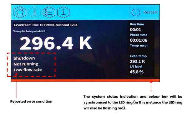
Figure 7.15 Home screen after system has shut-down with error
