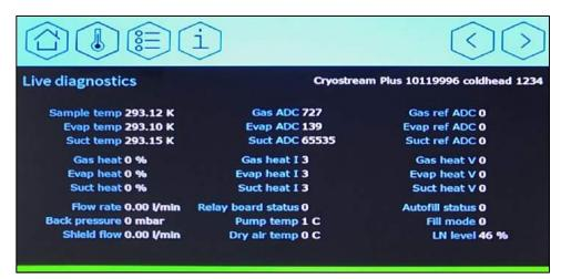
Figure 7.14 Info screen 1: Sensors and heaters
