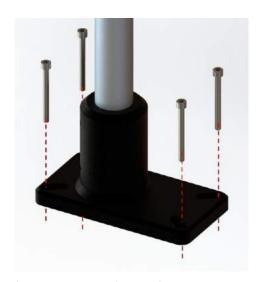
Figure 6.4 Schematic of varibeam base plate
