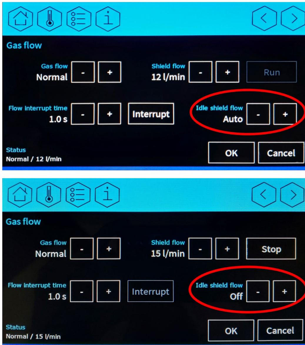
Figure 4 - Idle shield flow
