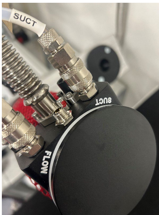
Figure 1 – Removing the gas hose from the FLOW line.
