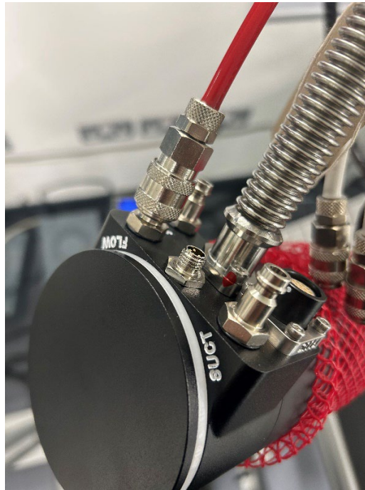
Figure 2 – Connecting the Dry-Air Inlet
